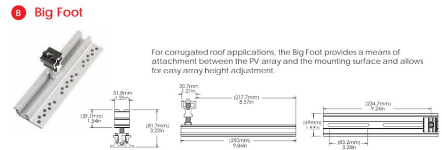
For corrugated roof applications, the Big Foot provides a means of attachment between the PV array and the mounting surface and allows for easy array height adjustment.
