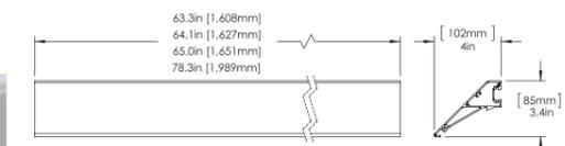
Enhancing both function and aesthetics, the Array skirt facilitates easy front-row installation while providing a clean look at the front of the PV array (available in both clear and black finish).
