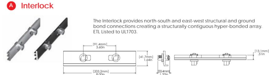
The Interlock provides north-south and east-west structural and ground bond connections creating a structurally contiguous hyper-bonded array. ETL Listed to UL1703.
